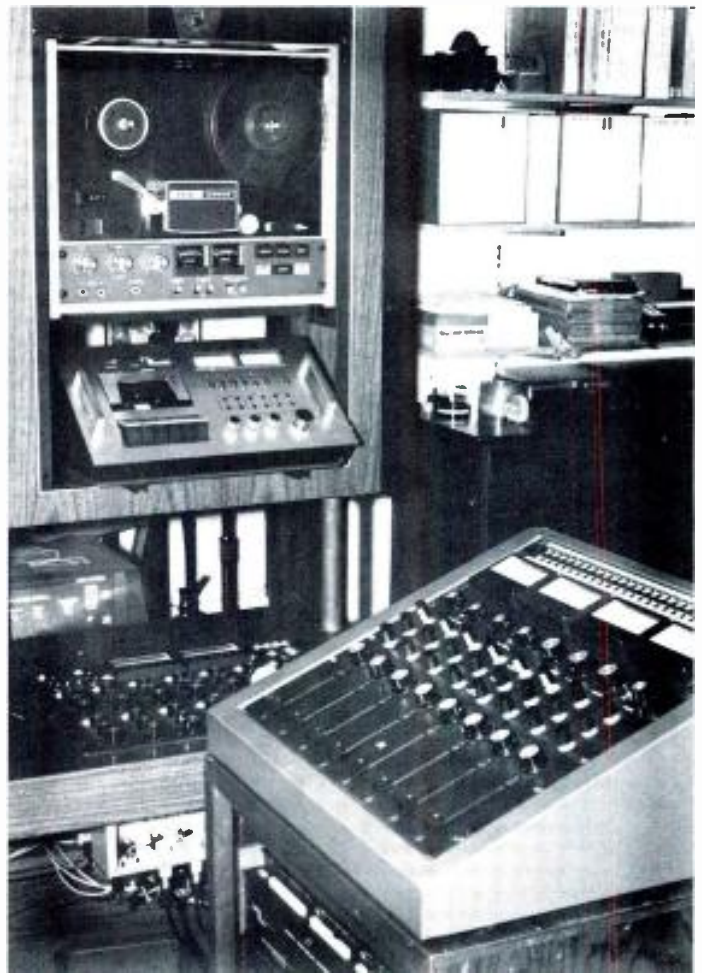
Another view of the control room, showing the front panel of the 8-channel, home-built, monitoring console.
